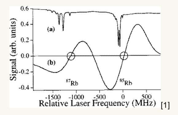
As can be seen, DAVLL offers a larger recapture range at the expense of slope. At the same time DAVLL is simpler, cheaper, and requires less support electronics.
