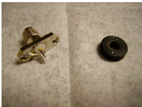
Figure 3: Step 3: Desolder the VCSEL from the SMA connector.
