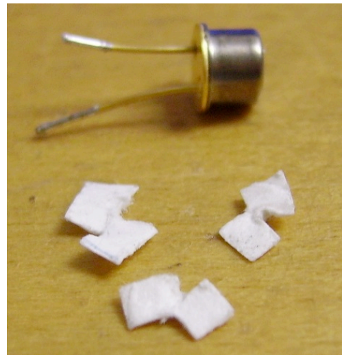
Figure 7: Step 6: Corners cut out of the square.
