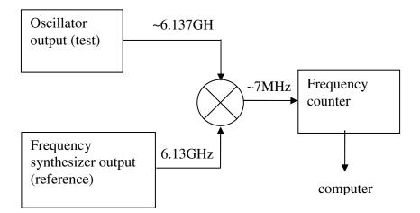
The oscillator was placed in an aluminum box to remove some of the parasitic electric signals, but no effort for temperature stabilization of the system was made. As a result we found that the long-term stability of the oscillator is determined by the temperature fluctuations in the room. *During these measurements we found that it is important to operate with external frequency reference feed into the counter – looks like the local frequency reference is defective.*
