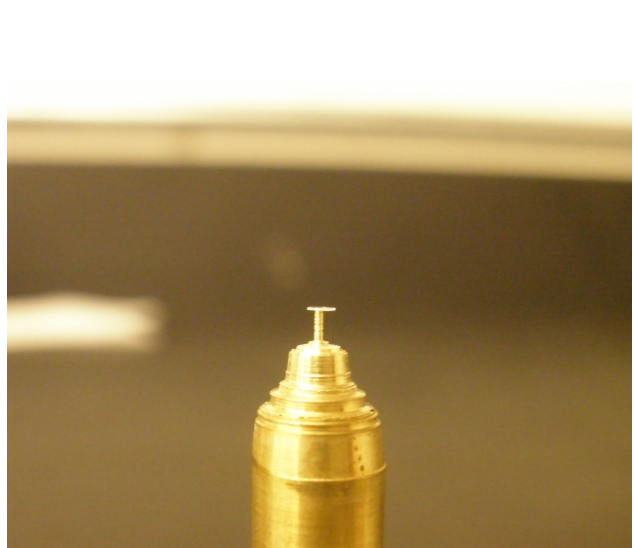
(d) A Lithium Niobate WGMR, 1.6mm in diameter (Polished by JPL, Q \simeq 5 \times 10^7 )
