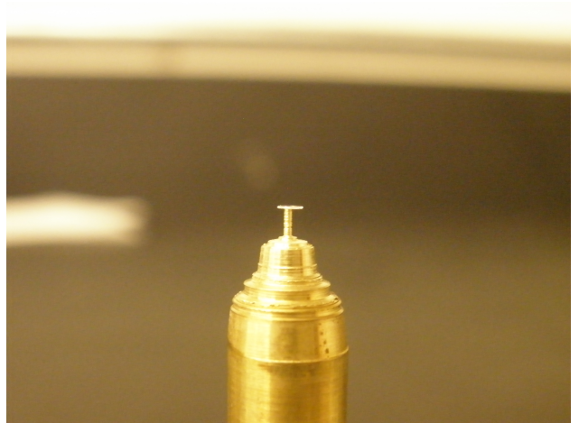
(d) A Lithium Niobate WGMR, 1.6mm in diameter (Polished by JPL, Q \simeq 5 \times 10^7 )
