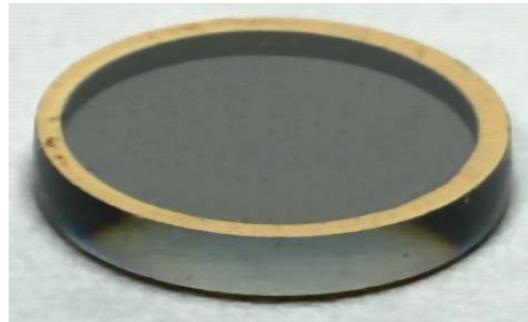
**Figure 15.** Photograph of a with radius  $R = 3 \text{ mm}$  and thickness  $d = 0.74 \text{ mm}$  z-cut  $\text{LiNbO}_3$  disk-shaped resonator with optically polished curved side-walls. Gold electrodes are placed in an annulus around the disk to increase the overlap of RF and optical fields.
